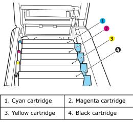
It will be necessary to remove the four image drums to gain access to the paper path.
